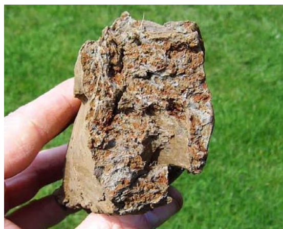
Red mottles in clay can indicate seasonal water logging and the need for land drainage
