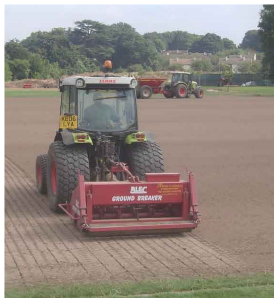
Alleviation of soil compaction can greatly improve the condition of natural turf facilities
