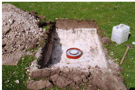
An investigation of the infiltration on the site is necessary to inform the design of the natural turf facilities
